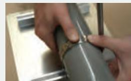
4. Hold down any excess band while finally tightening.
