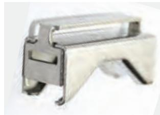
Two piece design features a saddle that slides into the sign channel. The saddle accepts all bands up to 19mm (3/4") and as the band tightens the saddle clamps tightly against the channel holding the sign securely in place.
