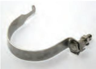
Simple sign installations are achieved by inserting the 'foot' into the sign channel, and twisting the clip through 90°. The other end is then secured by the bolt. Raised lips on the inner help prevent sign rotation.
